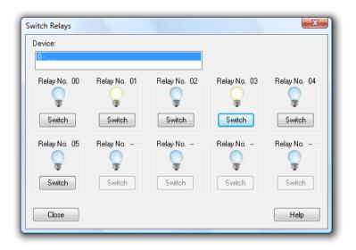
After selecting a device, the current status of the connected relays are displayed and can be changed with one mouse click, with the left mouse button, on the button "Switch". *Close* will close the dialog, *Help* will show this text.
