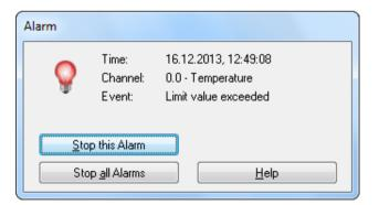
This message contains the time of the alarm, the channel that triggered the alarm and the event. It is possible to confirm only the displayed alarm or all alarms that occurred up until that moment.
