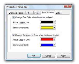
In the same way, the option "Change Background Color when Limits are violated" and the buttons on the lower frame can be used to select background colors.
